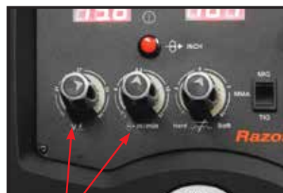
(19) Set welding parameters using the voltage and wire feed controls.
