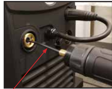
(12) Carefully feed the Polymide liner into the inlet guide tube hole of the torch euro receptacle
