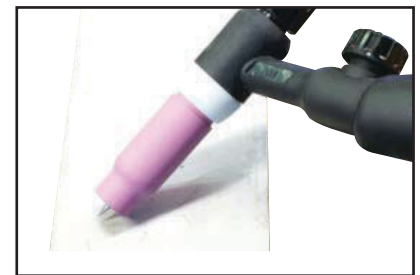
10) Lay the outside edge of the Gas Cup on the work piece with the Tungsten Electrode 1- 2mm from the work piece.
