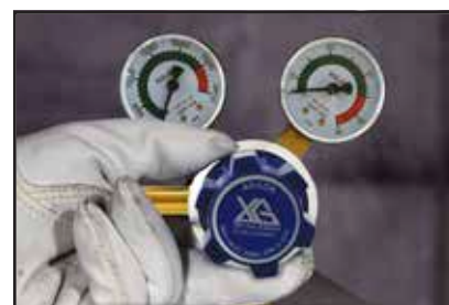
14) Carefully open the valve of the gas cylinder, set the flow to 6-10 l/min
