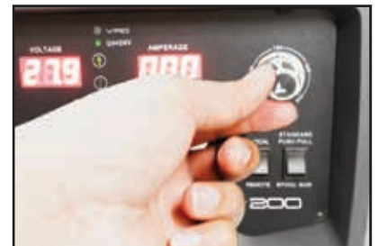
7) Set the welding current using the amperage control dial.
