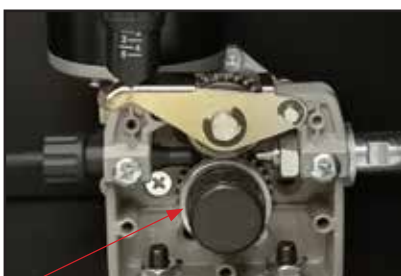
(6) Fit the correct type and size of drive rollers. V Groove for Hard Wires. Knurled for Flux Cored. U Groove for Aluminium.
