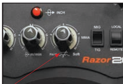
16) Set Inductance control to desired arc characteristic. Hard for tight narrow arc and Soft for wider softer arc. Half way is a good beginning position for most wires.
