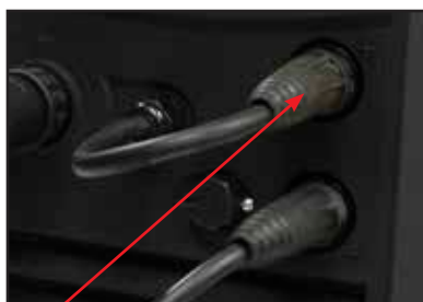
6) Connect weld power lead to \oplus Connect earth lead to \ominus
