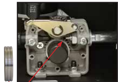
(9) Install a U groove drive roller of the correct size for the diameter wire being used.
