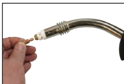
10) Remove the gas nozzle and contact tip from the front end of the mig torch.
