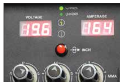
11) Press and hold the inch wire button to feed the wire down the torch cable through to the torch head.
