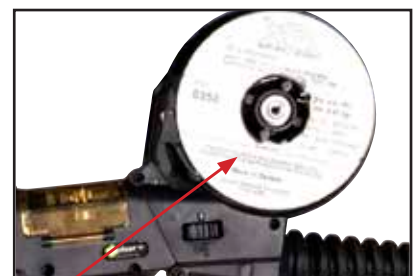
8) Place a spool of wire onto the Spool holder. Note: the spool retaining nut is Left Hand thread, turn it clockwise to undo it.
