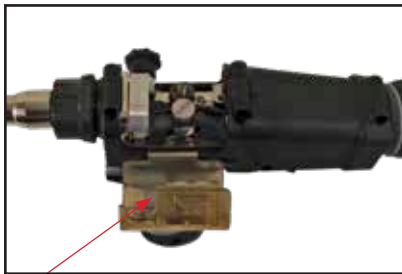
(9) Unclip and open the wire feed housing cover
