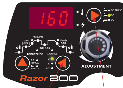
(2) Select DC Tig Function. Push the button until the DC icon illuminates green. Select 2T or 4T trigger function as required by the pushing the button to cycle through the trigger options. The icon will illuminate green for the selected trigger option.
