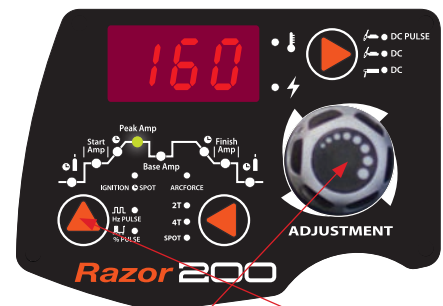
(3) Set the amps required by pushing the button, cycle through to illuminate the Peak Amp icon. Set the amperage with the encoder adjustment knob.
