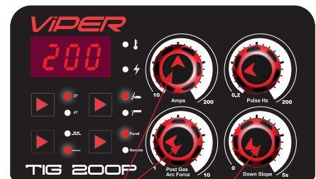
(3) Set the amps required by turning the amps adjustment knob. Set the downslope time and post gas time using the appropriate adjustment knobs.
