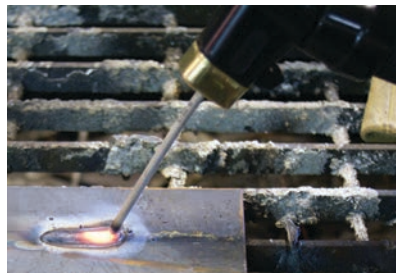
10) To finish the weld, break the arc by quickly snapping the electrode away from the work piece.
