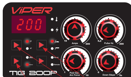
(2) Select DC TIG Function. Push the button until the DC icon illuminates red. Select 2T or 4T trigger function by the pushing the button to cycle through the trigger options. Select DC non pulse or pulse
