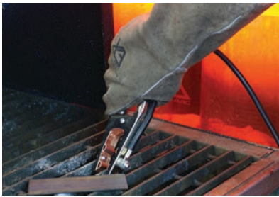
6) Connect the Earth Clamp securely to the work piece or the work bench.
