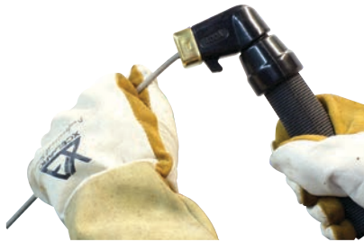
7) Place the electrode into the electrode holder and clamp tight.
