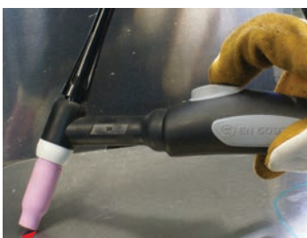
(4) Lay the outside edge of the Gas Cup on the work piece with the Tungsten Electrode 1- 3mm from the work piece
