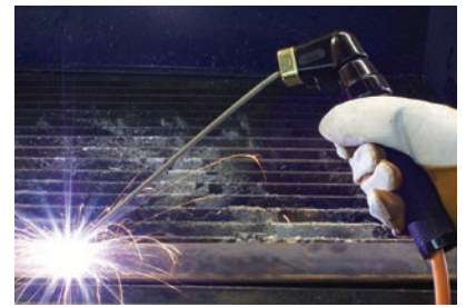
8) Strike the electrode against the work piece to create an arc and hold the electrode steady to maintain the arc
