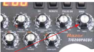
(2) Set the Peak Current at 110 Amps
