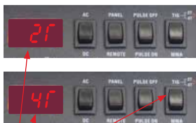
(10) Switch to the TIG function and the machine indicates what mode it is currently on (2T or 4T). To change the mode, switch off to MMA mode and back to TIG. Select 2T or 4T trigger function as required.
