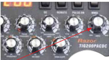
(2) Set the Peak Current at 110 Amps
