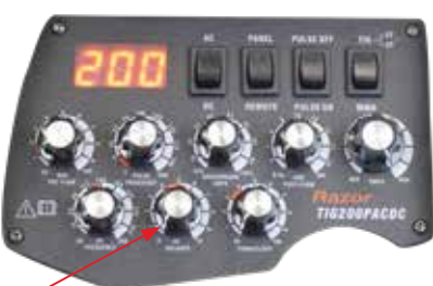
(12) Set the AC Balance knob between 4 & 5.
