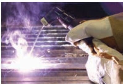
6) Hold the electrode slightly above the work piece to maintain the arc while travelling at an even speed to create and even weld deposition.
