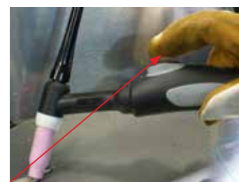
(6) Release the torch switch to bring in the end of the welding sequence dependant of 2T or 4T trigger function choice
