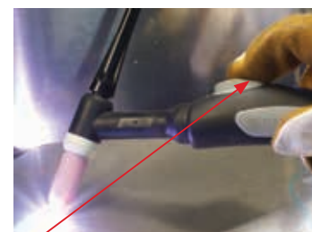
(14) Press the torch switch and the arc will ignite across the gap between the tungsten and work piece. Hold even distance of about 2mm gap between the tungsten and work piece to maintain the arc.
