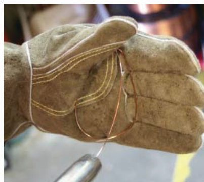
(8) A simple check for the correct drive tension is to bend the end of the wire over hold it about 100mm from your hand and let it run into your hand, it should coil round in your hand without stopping and slipping at the drive rollers, increase the tension if it slips.
