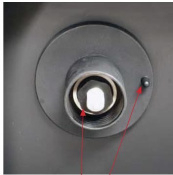
(2) Note the tension spring adjuster and spool locating pin.
