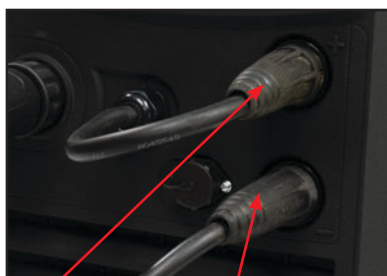
6) Connect weld power lead to ⊕ Connect earth lead to ⊖
