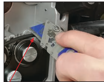
(15) Cut the extended liner with a sharp Stanley knife just in front of the drive roller,
