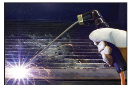
5) Strike the electrode against the work piece to create an arc and hold the electrode steady to maintain the arc
