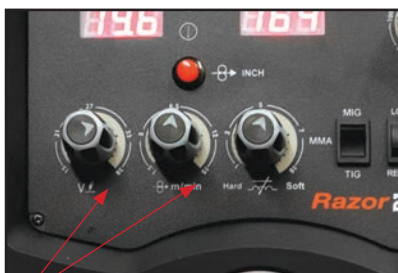
(16) Set welding parameters using the voltage and wire feed controls.
