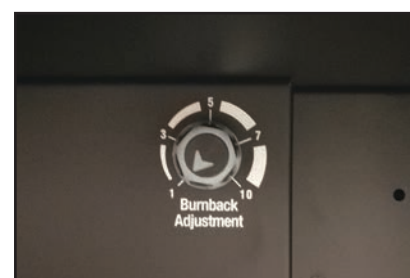
17) Adjust the burn back control to prevent the wire sticking in the weld pool. Burn back control is located above the wire feed motor.
