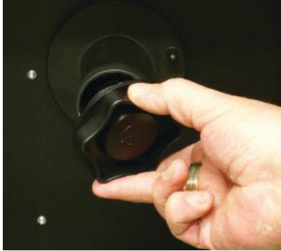
(1) Remove the spool retaining nut.
