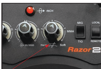
16) Set Inductance control to desired arc characteristic. Hard for tight narrow arc and Soft for wider softer arc. Half way is a good beginning position for most wires.
