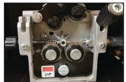
8) Feed wire over the drive roller into the outlet guide tube, Push the wire through approx 150mm.
