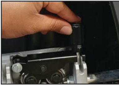
9) Close down the top roller bracket and clip the pressure arm into place. Apply a medium amount of pressure to the drive roller.
