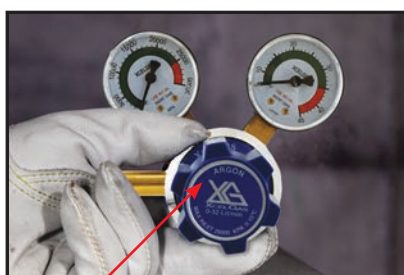
(18) Carefully open the valve of the gas cylinder, set the flow to 12-15 l/min
