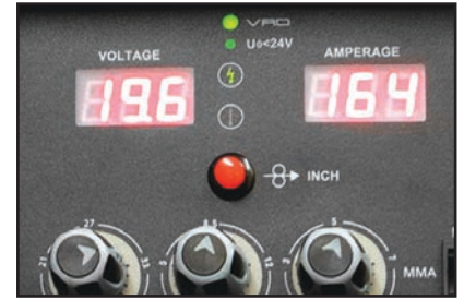
11) Press and hold the inch wire button to feed the wire down the torch cable through to the torch head.
