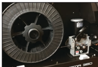
7) Place wire onto spool holder - (spool retaining nut is left hand thread ) Feed the wire through the inlet guide tube into the drive roller.
