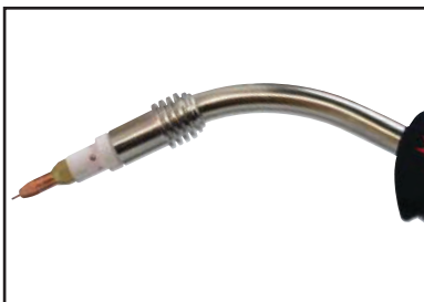
12) Fit the correct size contact tip over the wire and fasten tightly into the tip holder.
