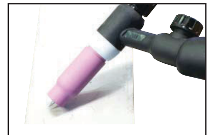
10) Lay the outside edge of the Gas Cup on the work piece with the Tungsten Electrode 1- 2mm from the work piece.
