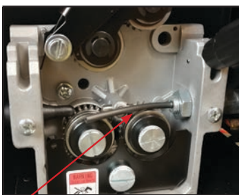
(13) Take the extended Polymide liner all the way up and over the drive roller
