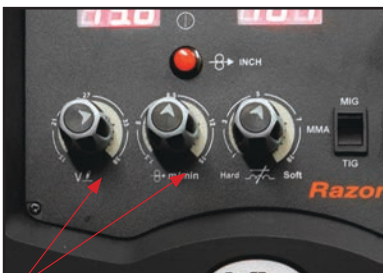
15) Set welding parameters using the voltage and wire feed controls.
