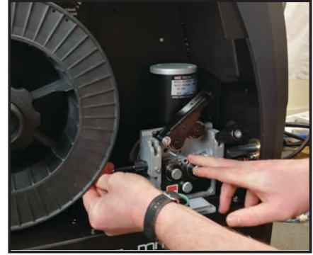
(3) Snip the wire carefully, be sure to hold the wire to prevent the spool uncoiling.
