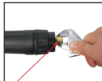
(9) Fully screw down the liner retaining nut and nip it up tight.
