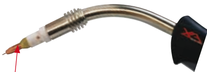
(12) Fit the correct size contact tip over the wire and fasten tightly into the tip holder.
