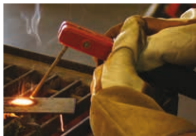
7) To finish the weld, break the arc by quickly snapping the electrode away from the work piece.
