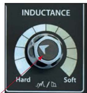
(17) Set the inductance with the front panel control knob. Less inductance for a tight hard arc, more inductance for a softer, wider arc.
