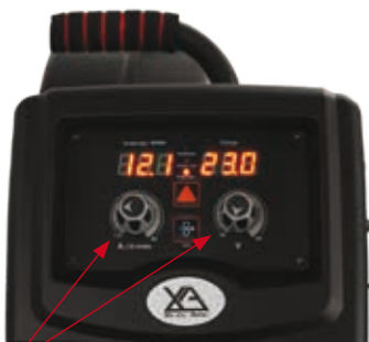
(15) Set welding parameters using the voltage and wire feed controls.
