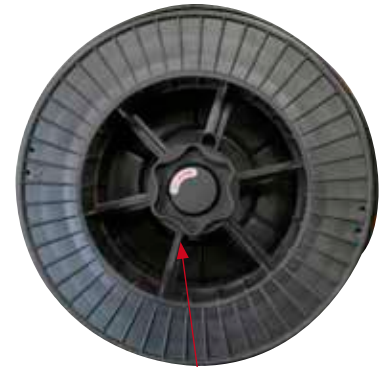
(3) Fit the wire spool onto the spool holder fitting the locating pin into the location hole on the spool. Replace the spool retaining nut tightly
