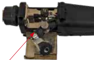
(10) Unclip and swing back the wire tension swing arm. Check the that the correct drive roller is installed.
