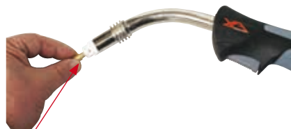
(8) Replace the front end parts
