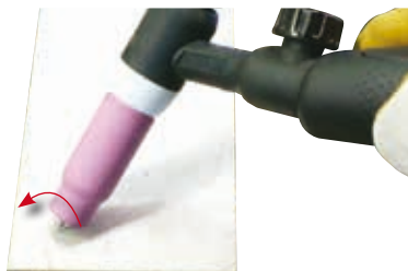
(8) With a small movement rotate the Gas Cup forward so that the Tungsten Electrode touches the work piece.
