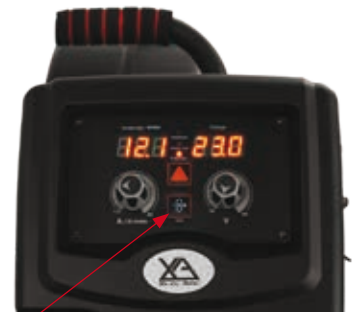
(11) Press and hold the inch wire button to feed the wire down the torch cable through to the torch head.
