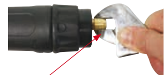
(9) Fully screw down the liner retaining nut and nip it up tight.
