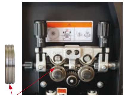
(9) Install U groove drive rollers of the correct size for the diameter wire being used.
