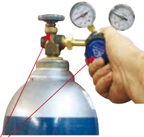
(6) Carefully open the cylinder gas valve, set the flow to between 6-10 l/min
