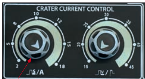
(4) Set the welding current using the amp control dial
