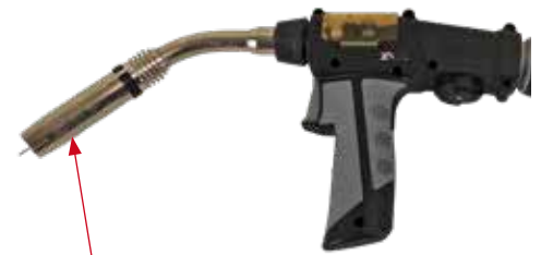
(14) Fit the gas nozzle, close the wire feed housing cover ready for welding.
