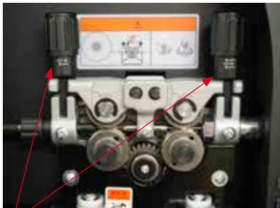
(9) Close down the top roller bracket and clip the pressure arm into place. Apply a medium amount of pressure to the drive roller
