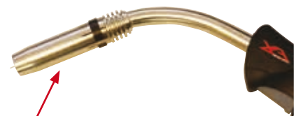
(18) Fit the remaining front end parts to the torch neck ready for welding.
