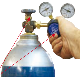
(15) Carefully open the valve of the gas cylinder, set the flow to 12-18 l/min
