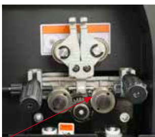
(6) Fit the correct type and size of drive rollers. V Groove for Hard Wires. Knurled for Flux Cored. U Groove for Aluminium.
