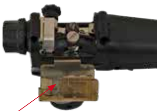
(09) Unclip and open the wire feed housing cover
