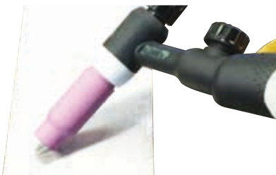
(7) Lay the outside edge of the Gas Cup on the work piece with the Tungsten Electrode 1- 2mm from the work piece.
