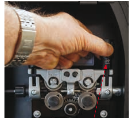
(6) Lock down the top pressure roller and apply a medium amount of pressure using the tension adjustment knob
