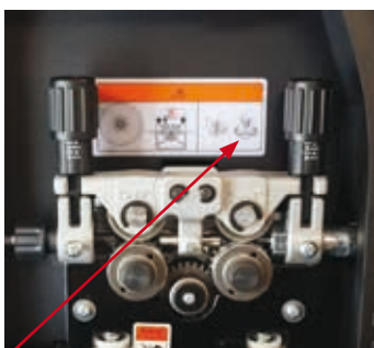
(16) Feed the wire through the drive rollers, apply light pressure on the drive rollers.
