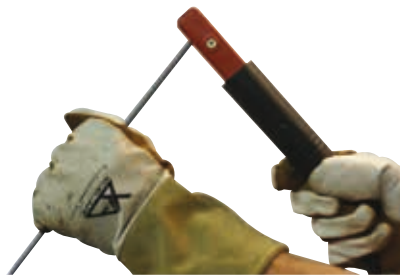
4) Place the electrode into the electrode holder and clamp tight.
