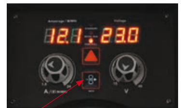
(11) Lay the torch cable straight or in a gentle curve on the floor. Use the inch button to feed the wire down the cable into the torch drive unit. Release the inch button when the wire reaches the torch drive unit.
