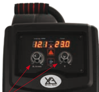
(16) Set welding parameters using the voltage and wire feed controls.
