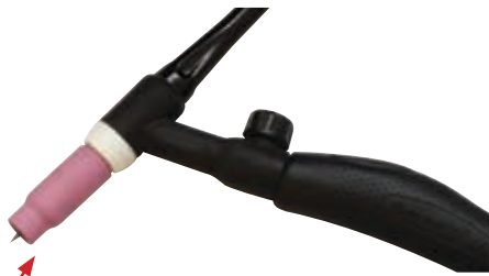
(8) Assemble front end parts of the TIG torch, fitting a sharpened tungsten suitable for DC welding.
