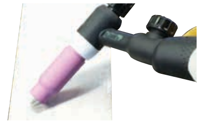
(10) Lay the outside edge of the Gas Cup on the work piece with the Tungsten Electrode 1- 2mm from the work piece.
