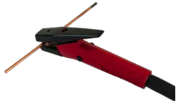
(8) Insert the Carbon between the jaws, the carbon should not extend too far out otherwise the air flow will not meet with the arc gouging zone at the workpiece.
