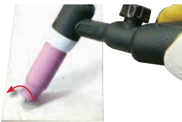
(11) With a small movement rotate the Gas Cup forward so that the Tungsten Electrode touches the work piece.
